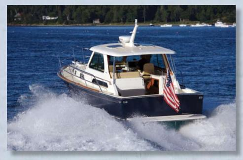
Sabre is well known for creating yachts that are safe, practical and functional. The Sabre 34 Hard Top Express is no exception, with sturdy 1.25 inch diameter perimeter rails and additional handrails provided beneath the overhang of the hard top. Wide side decks and teak toe rails offer secure footing when moving from cockpit to foredeck for anchoring and docking procedures. The molded anti-slip surface provides additional security on deck.
