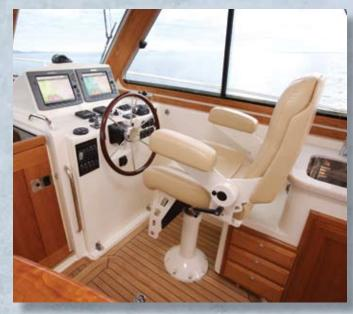
The helm pod has ample space for multiple LCD screens, other navigational devices and all engine controls. The wood trimmed wheel is another elegant feature of the helm area. Large forward windows and sliding side windows allow a full view ahead and alongside the yacht, and heavy duty windshield wipers and washers will keep the view clear in poor conditions. Site lines are excellent and meet ABYC recommendations. Bow rise at cruise speed is less than five degrees.
